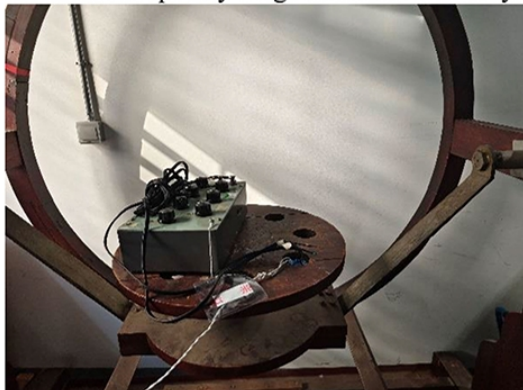
Industrial frequency magnetic field immunity test photo:
