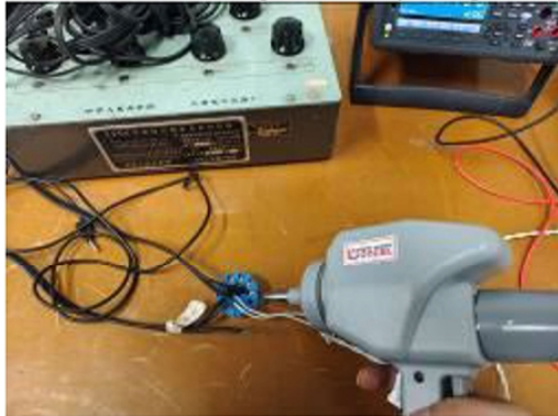
Electrostatic discharge immunity test photo:
