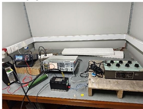
Conducted Harassment Immunity Test Photographs for RF Field Induction:
