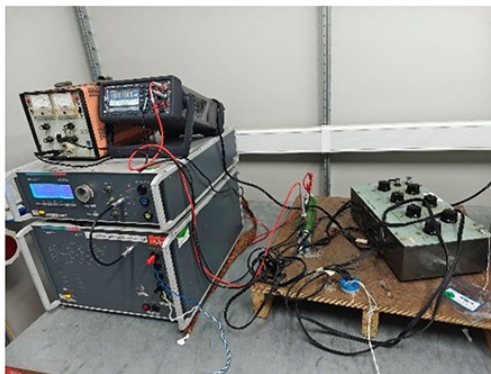
Industrial frequency magnetic field immunity test photo:
