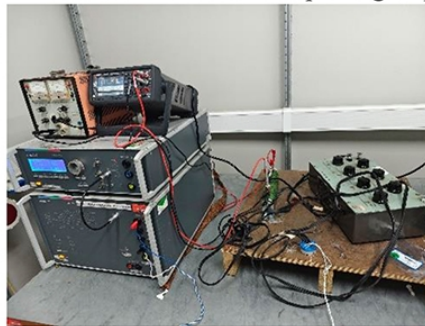
Electrical fast transient pulse group immunity test photo:
